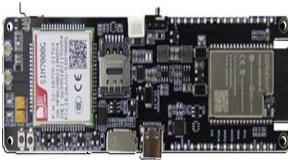
Figure 1: LILYGO T-SIM7000G development board
