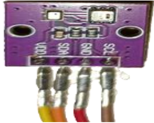
Figure 2: BME280 sensor (for temperature, pressure and relative humidity)
