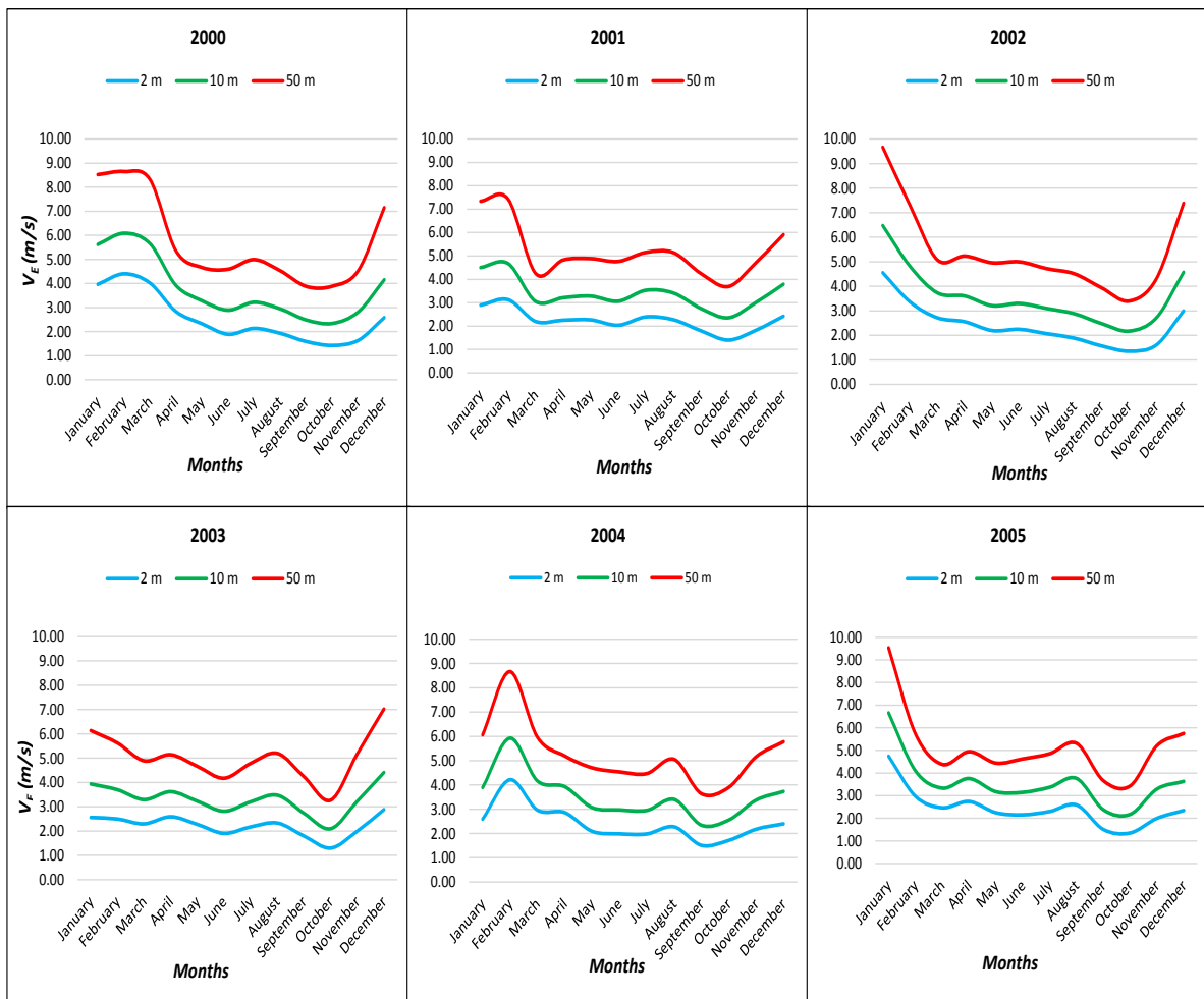
Figure 7: Wind speed carrying maximum energy, V_E plot at different heights for 6 years
