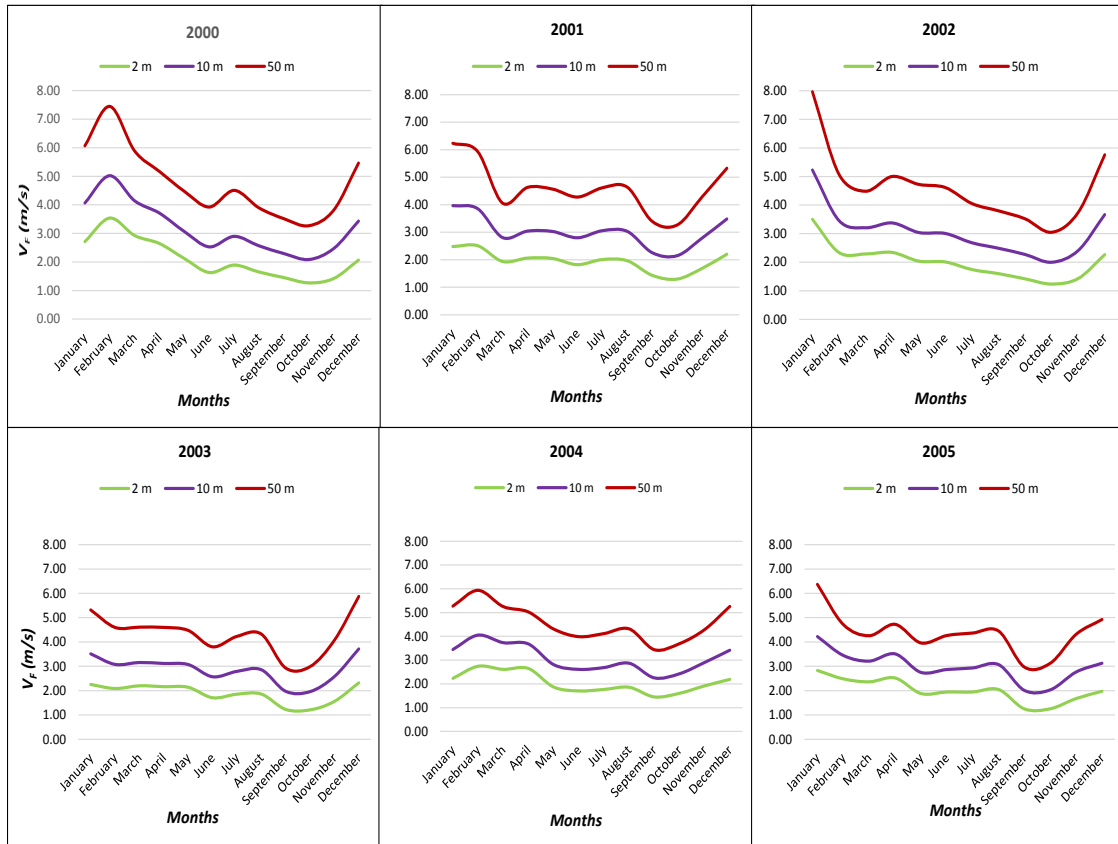
Figure 6: Most probable wind speed, V_F plot at different heights for 6 years
