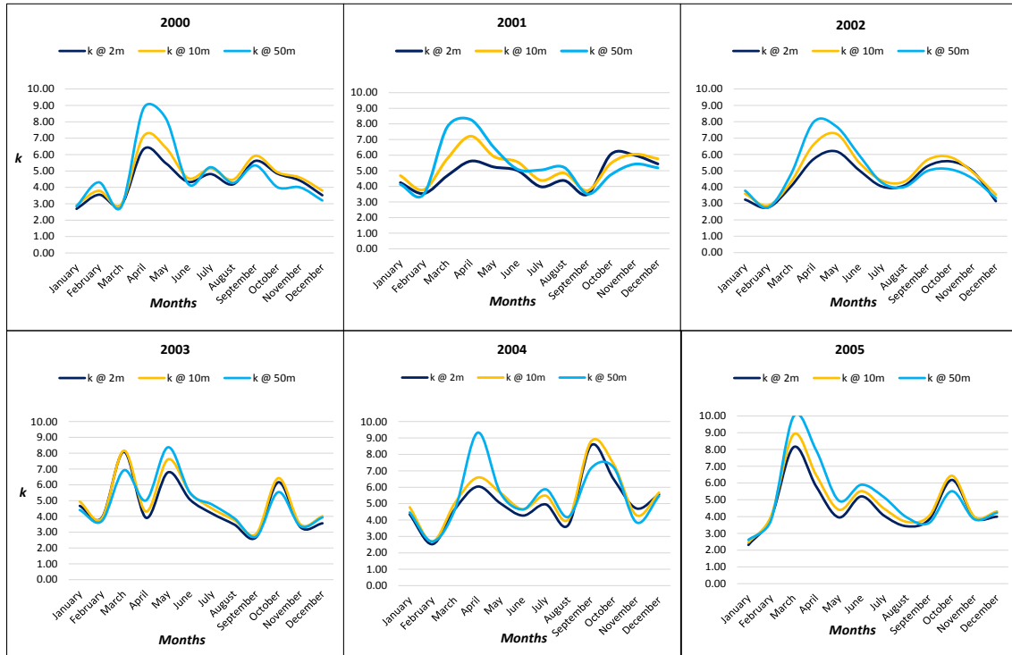
Figure 4: Weibull shape parameter, k plot at different height for 6 years (2000 – 2005)
