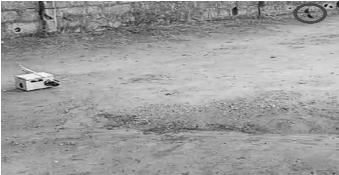
Figure 7: Open-field test demonstrating successful avian flight response (highlighted by the black circle) upon system activation
