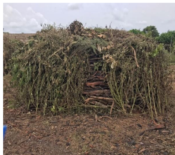
Figure 2: Earth-mound charcoal kiln
