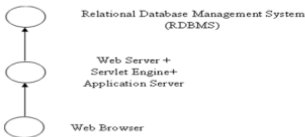
Figure 10: Three-tier architecture model
