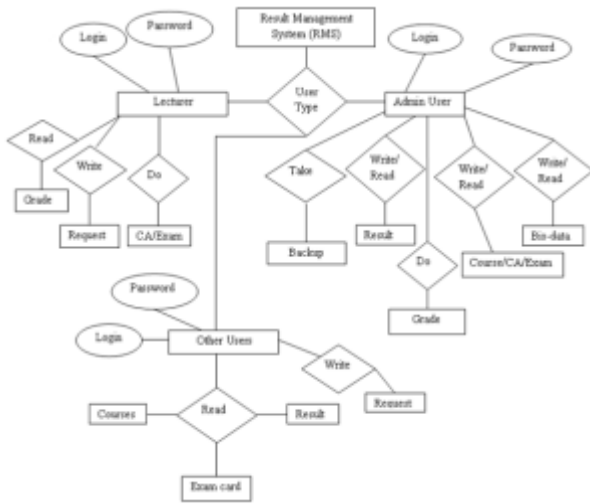
Figure 5: Proposed Examination Management System Entity Relational Diagram
