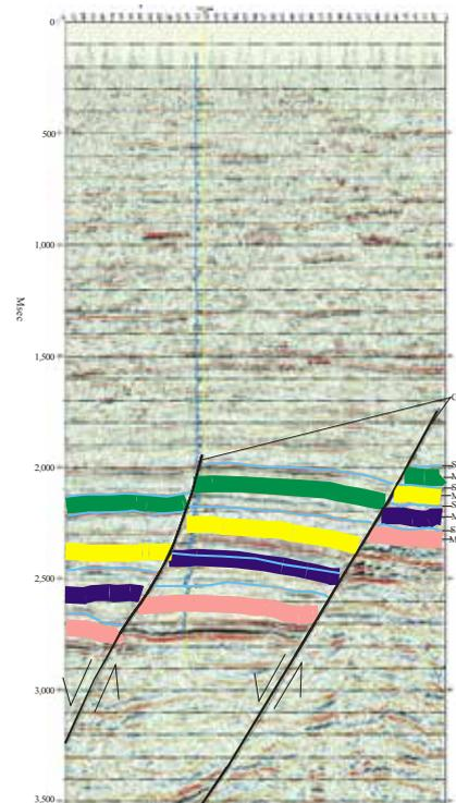
Fig. 11. Structures with growth faults along cross-line (strike) 1,600
