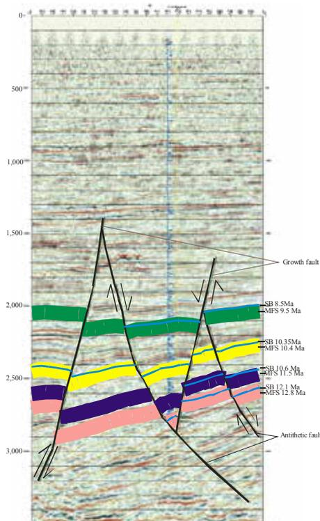
Fig. 9. Collapsed crest structures and fault styles and throw along in-line (dip) 5,980 section
