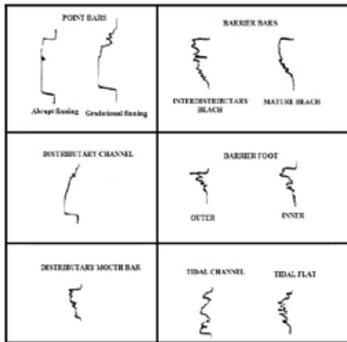
Fig. 7. Gamma Ray Log Stacking Patterns Defining Deltaic Depositional Environments (Source: Schlumberger, 1985)
