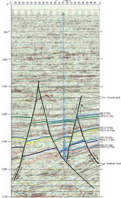
Fig. 8. Interpreted seismic section showing transect along in-line (dip) 5,980 section
