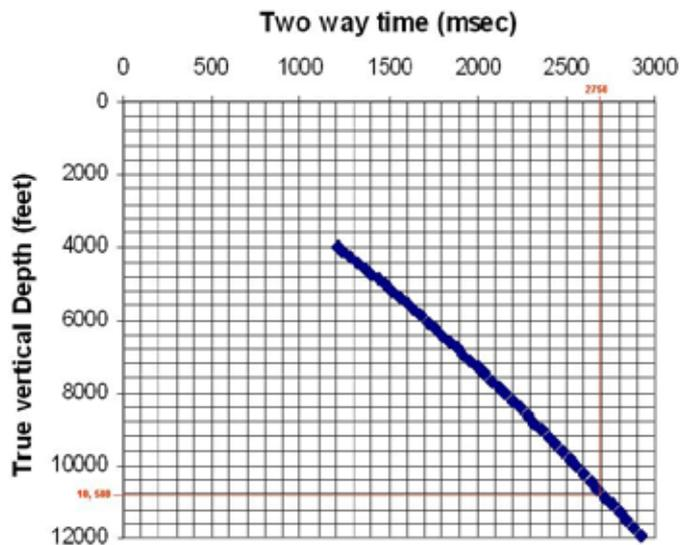
Fig. 5. The Plot of Check Shot Chart for TMB-1 Well (Conversion: 1 foot = 0.3048 metre)
