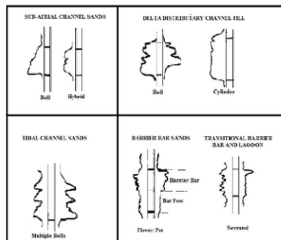
Fig. 6. Gamma Ray and Resistivity Log Patterns Indicative of Depositional Environments (Source: Busch, 1975)
